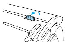
6 With the lower part of the stand between the handle and machine, slide the spool stand to the left so that the pin fits into the hole in the machine, and then fit the spool stand into the latch.
